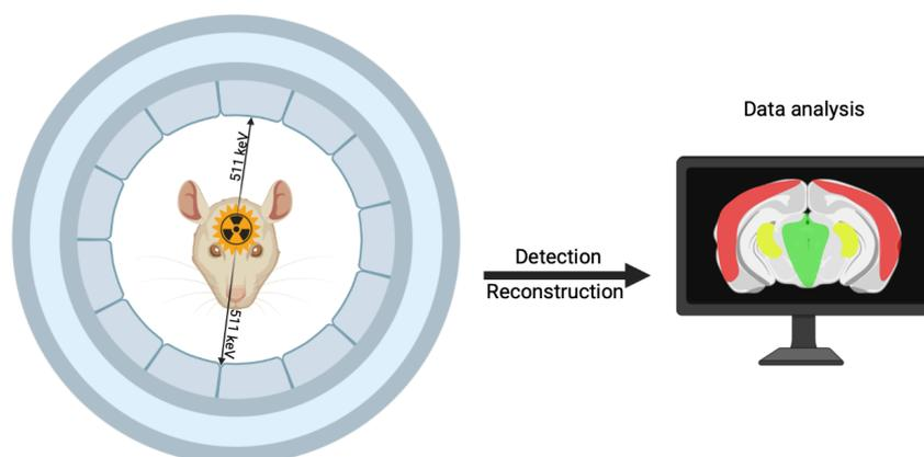
Figure 9: Simplified schematic view of the PET scanner principle. Created in biorender.com
